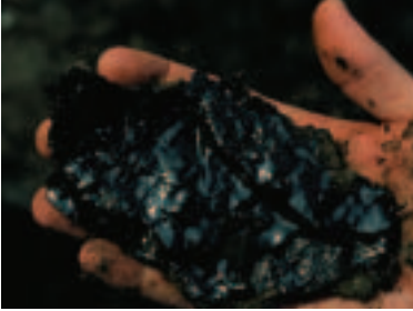
This sample of oil sands contains bitumen, which is a sticky black substance. Scientists had to find a way to separate it from the sand.
